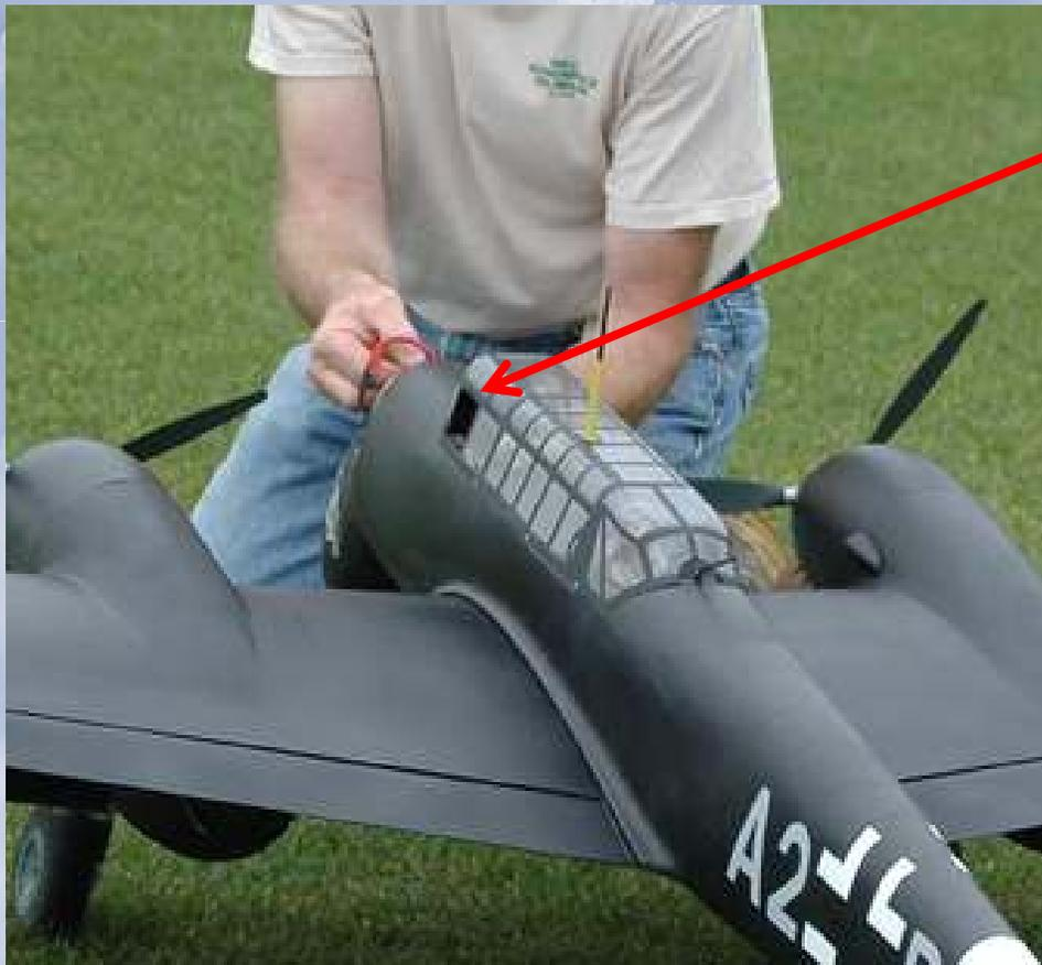
**Note side window of KMP (EMS) BF-110 is slid open to facilitate cooling of ESC's located just below window sill.**
