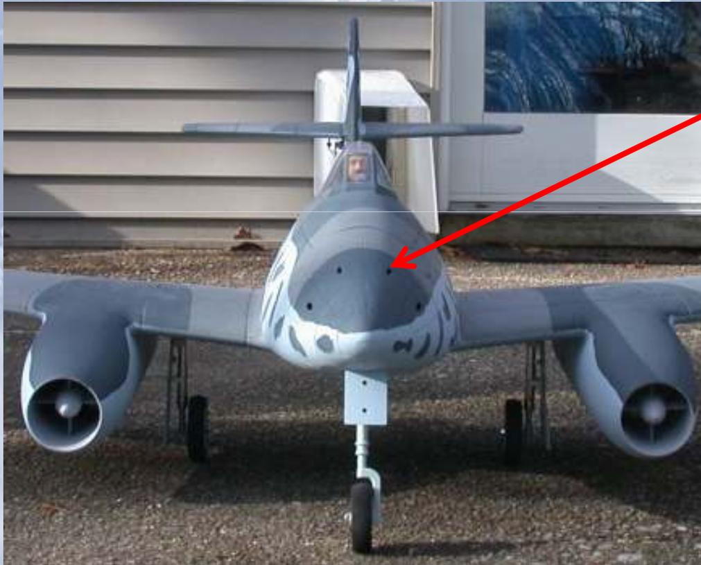
**Gun ports let air into fuselage just in front of battery
